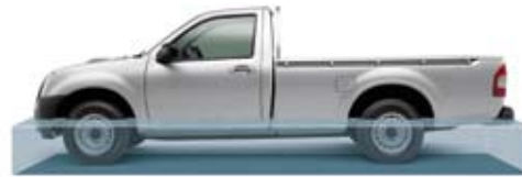
Wading depth 400mm @ 15km/h
