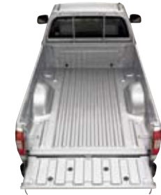
Load dimensions: Length 2,280mm Width 1,520mm Height 450mm (At highest point)
